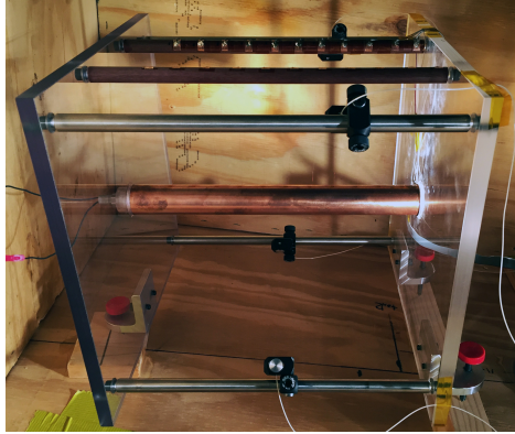
Figure 2: Cylinder test 8-1905 with the detonator at left, breakout window at right.
