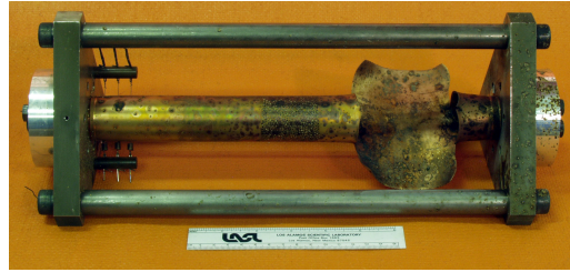
Fig. 3. Photo of a recovered shot assembly (Shot# 8-1032).
