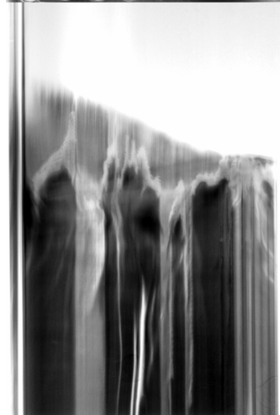
FIGURE 14. Streak data from a non-violent long slot test.
